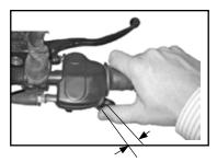
Measure the throttle lever play. 3.0~5.0mm (0.12~0.20in) as shown
