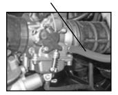
Inspect the fuel hose for damage and fuel leakage. If any defects are found, the fuel hose must be replaced.
