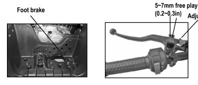
Rear hand brake located on left side of handlebar
