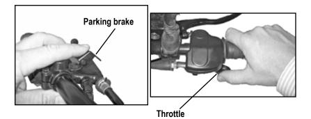
When you are sure that the engine is warm release parking brake. Release brake lever and open the throttle gradually to move forward.
