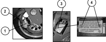
1. Inspect front disk brake caliper (1) for leakage. If brake fluid leaks, the safety of riding could be affected.
