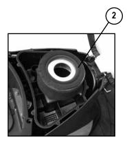
Air filter (2) is located under seat of scooter.
