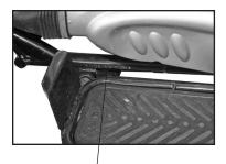
The frame number is stamped on the frame between the front wheels.
