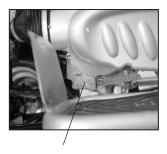
The engine number is stamped on the left side of the engine case below the cylinder.
