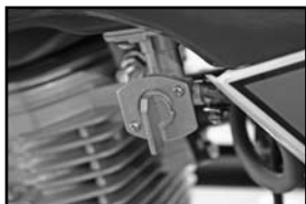
Fuel Valve ON
