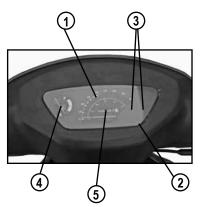
• Odometer (5): Indicates the total distance the vehicle has traveled, in km.
