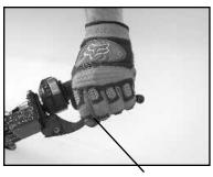
Rear Brake To stop the ATV, first release the throttle lever, then apply the rear and front brakes smoothly.
