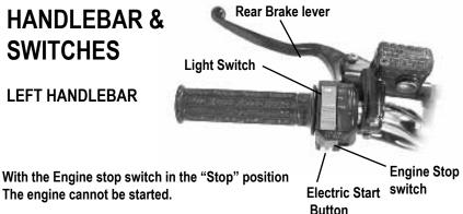
With the Engine stop in the "Run" position The engine can be started.
