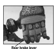
When you are sure that the engine is warm, release the rear brake.
