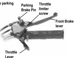
Use throttle adjusting screw to restrict maximum speed of ATV. Adjust this limiter according to rider's skill and experience.
