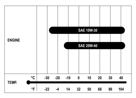
Use the chart to select a viscosity rating based on the temperature range in your area.
