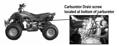
Before transporting the ATV make sure the fuel valve is turned to the off position then drain fuel from the carburetor as follows:
