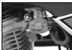
Fuel Valve OFF
